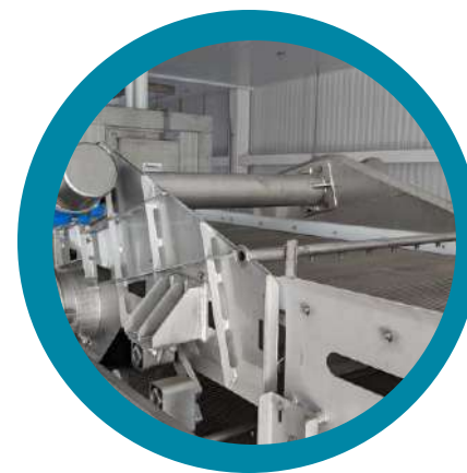
+ Dewatering (Fluid Removal System)
