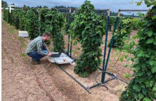
(A-E) Installation of the weighing lysimeters for 'Columbia Star' blackberry. (F) Crop evapotranspiration is measured continuously using data loggers.
