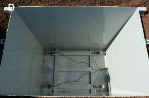
(A-E) Installation of the weighing lysimeters for 'Columbia Star' blackberry. (F) Crop evapotranspiration is measured continuously using data loggers.
