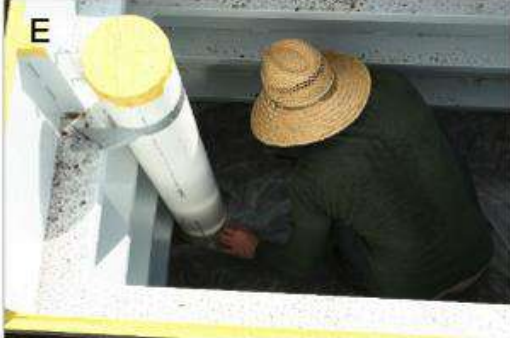
(A-E) Installation of the weighing lysimeters for 'Columbia Star' blackberry. (F) Crop evapotranspiration is measured continuously using data loggers.
